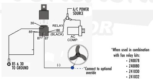
**NOTE:** If installing either (or both) an Auxiliary Switch or an Adjustable Temperature Controller with this A/C Relay, wire those items by tapping into the wire between the A/C Relay and the fan motor using 3-way connectors.
