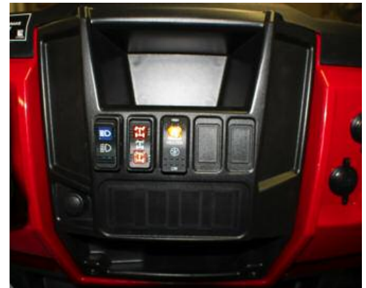
PHOTO 10: Switch mount center panel
