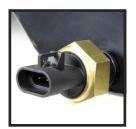
**Step 3:** This is an NPT fitting. Install the coolant level sensor finger tight into the port located in Step 1. Then, tighten 1.5 - 2.5 more turns with a wrench.
